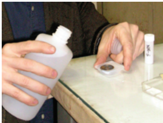
Figure 1 The simple process of extracting lead from a silver ornament at the National Museum, Karachi, Pakistan, using an EDTA solution.
