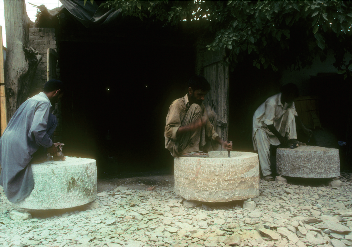
Figure 5.22 Workmen carving millstones out of Pab sandstone.
