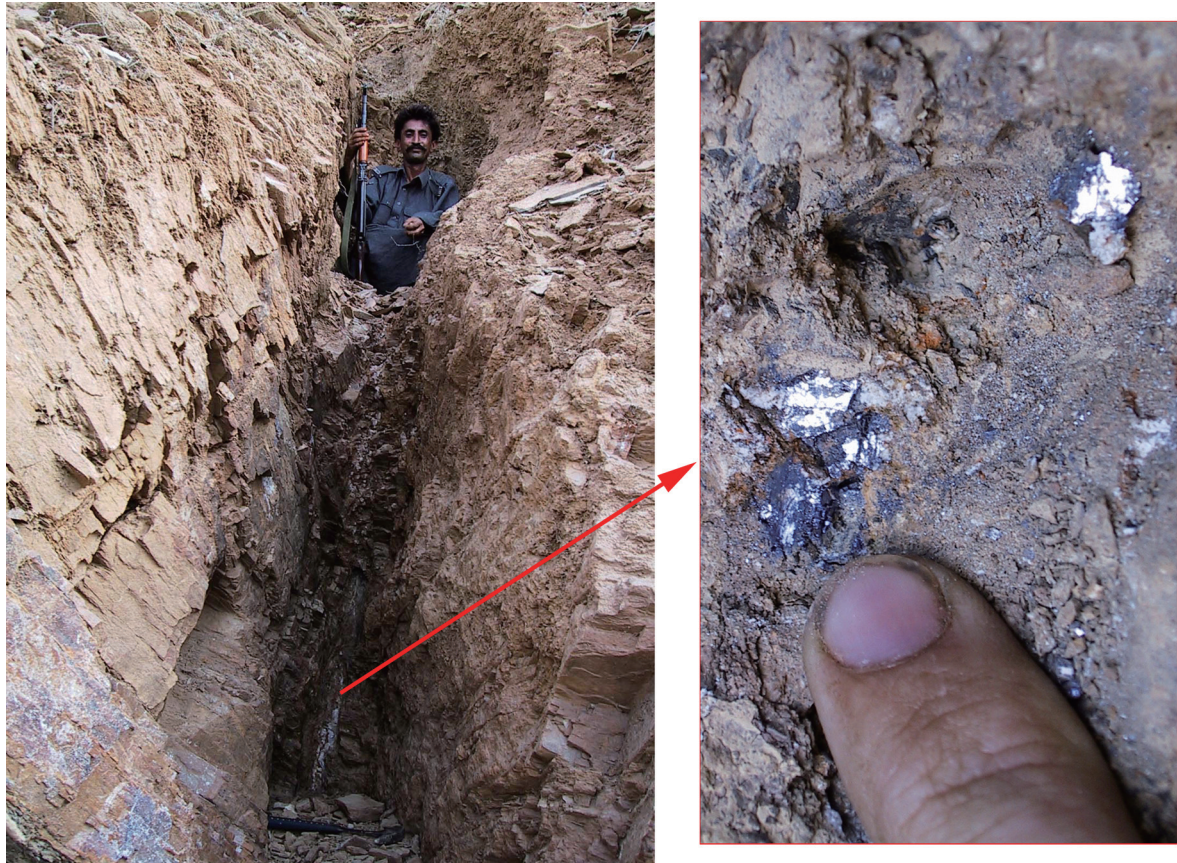
Figure 12.6 Sampling a galena seam at Bamph Nala, Kanrach Valley, Balochistan.
