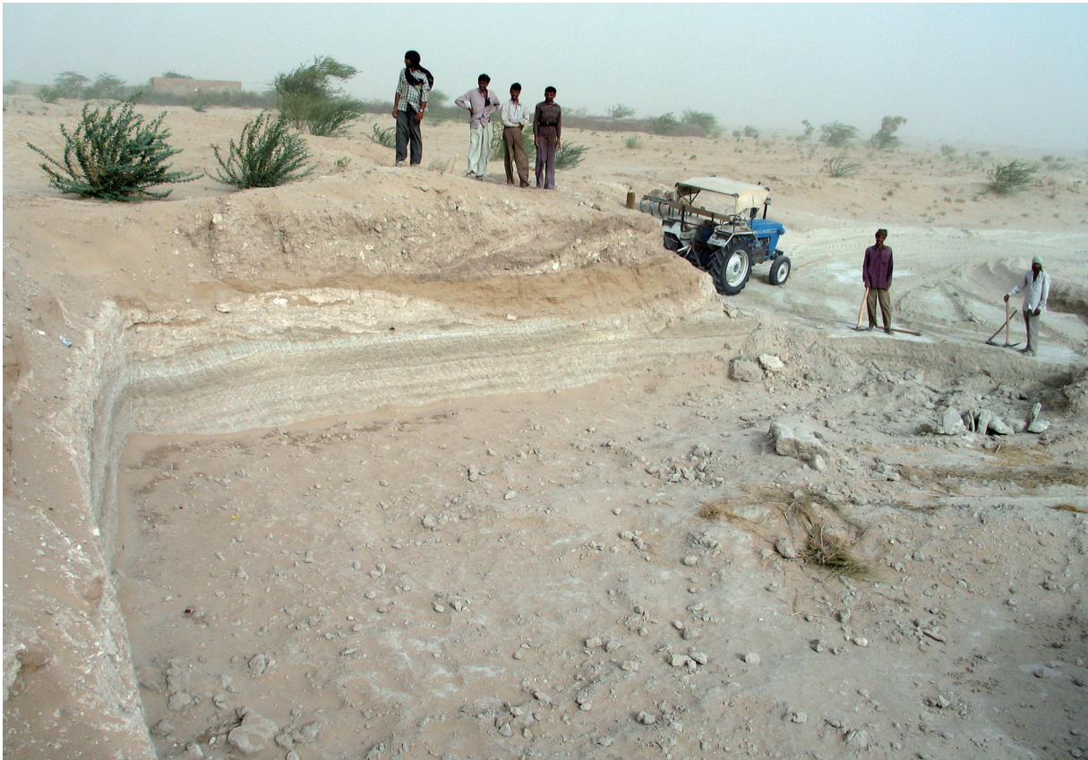
Figure 10.6 Quaternary gypsite deposit immediately below the desert alluvium, Bikaner district, western Rajasthan.
