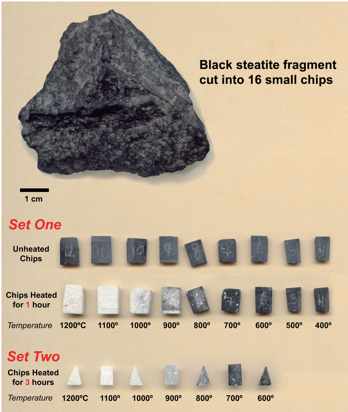
Appendix 7.12 Figure 1 The black steatite fragment from the MR4 atelier used in this experimental study (top) and the two sets of chips cut from it before and after heating.
