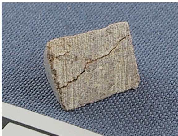
Appendix 7.16 Figure 5 Cracked tablet RRD (post-firing).
