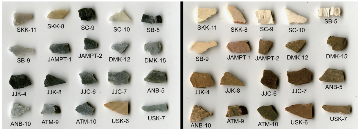
Appendix 7.17 Figure 1 Left - A set of chips taken from 20 geologic samples previously subjected to INAA. Right - The same 20 chips after being fired at 1200°C for one hour.
