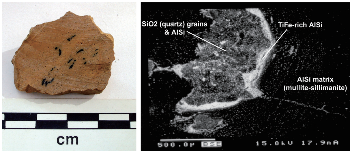
Appendix 4.5 Figure 4 “Ernestite” fragment H2000/2090-49 (left). BSE image of black patch (right).
